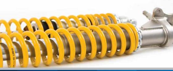
Single tube design/ McPherson strut
