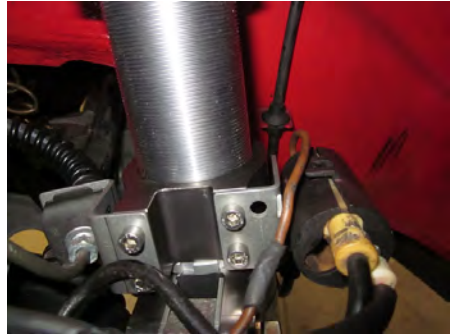
Fig. 1: Brake line and cable are mounted on the new attachments on the Öhlins strut.
